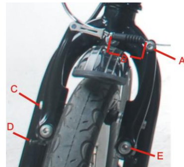
A-Cable clamp bolt B-No contact C-pad fixing bolt D-Centering screw E-Arm fixing bolt
